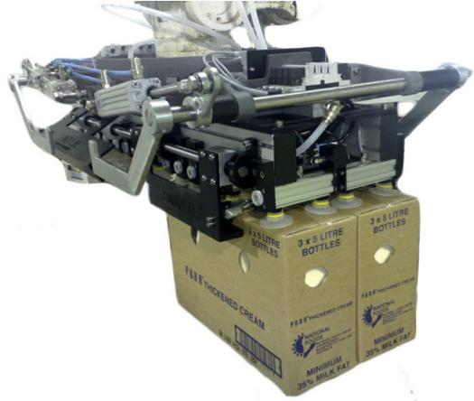
Specialised cups allow us to easily handle liquid filled bags, soft pouches, oily metal plus we have direct food contact cups that are metal detectable.
