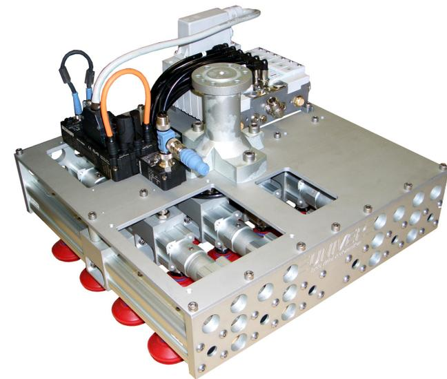
As Collaborative robots become more common we can supply a head that is light weight and includes the generator, valves, a display etc.
